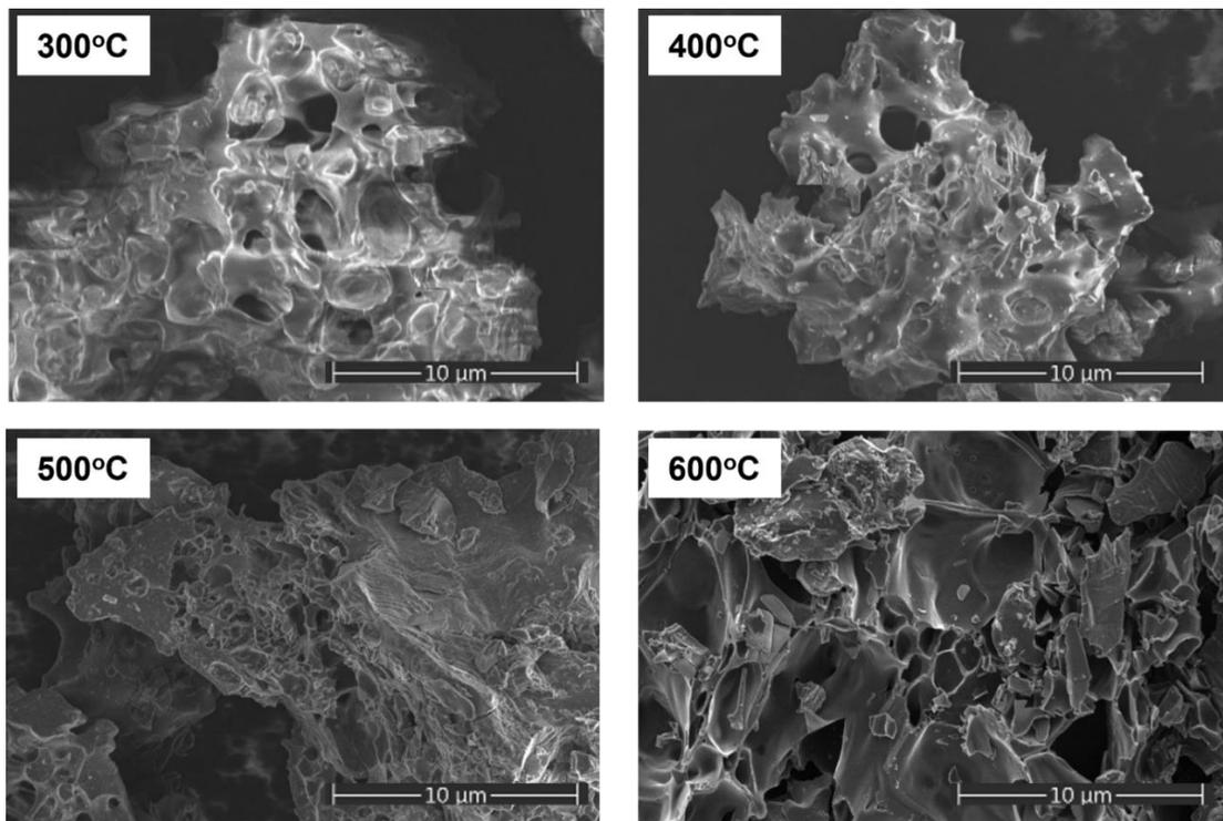
**Figure 2.** Effect temperature of pyrolysis on the surface morphology of durian seed biochar. Figures (a), (b), (c), and (d) are samples heated at 300, 400, 500, and 600°C.
