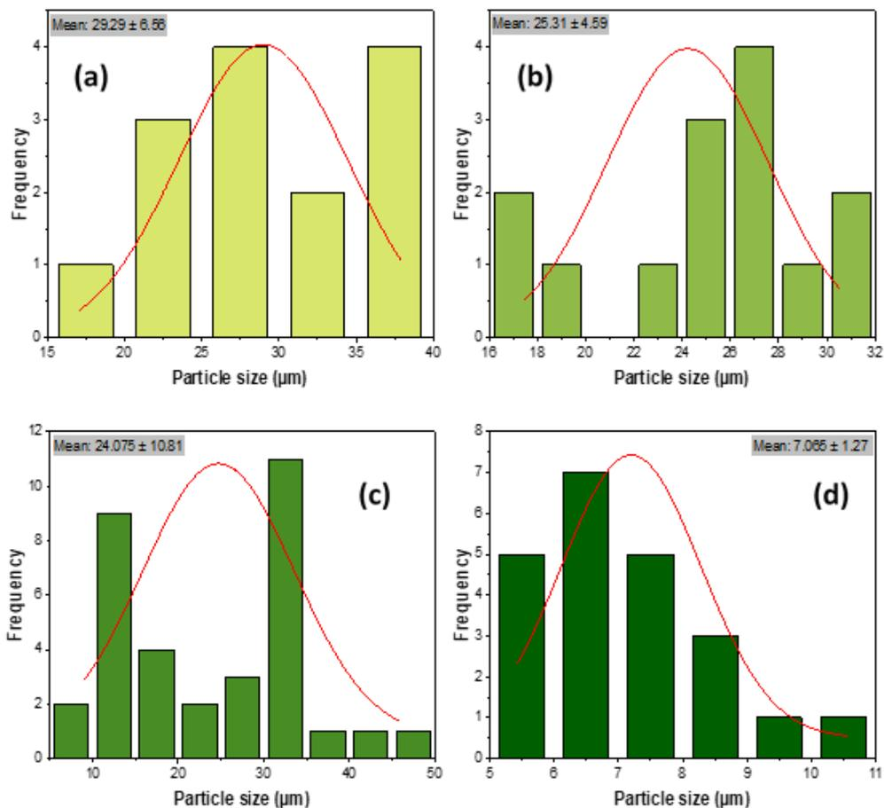
**Figure 3.** Particle size distribution at (a) 300oC, (b) 400oC, (c) 500oC, and (d) 600oC.
