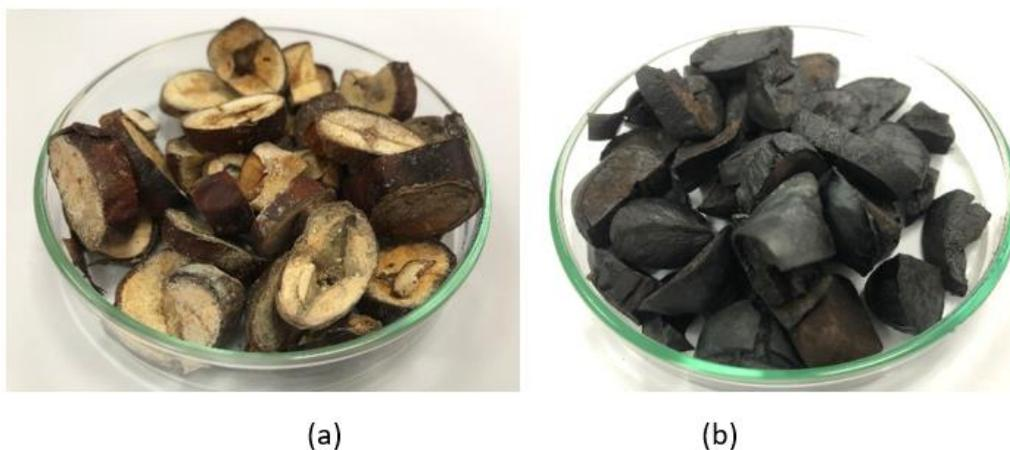
**Figure 1.** Raw material (a) and biochar after pyrolysis (b).
