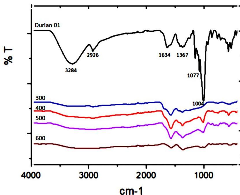
**Figure 4.** Raw material durian dan biochars FTIR spectrum.
